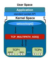
Fig. 2. Creation of new subflows using the API.
