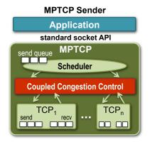
Fig. 1. TCP stack with MPTCP support.
